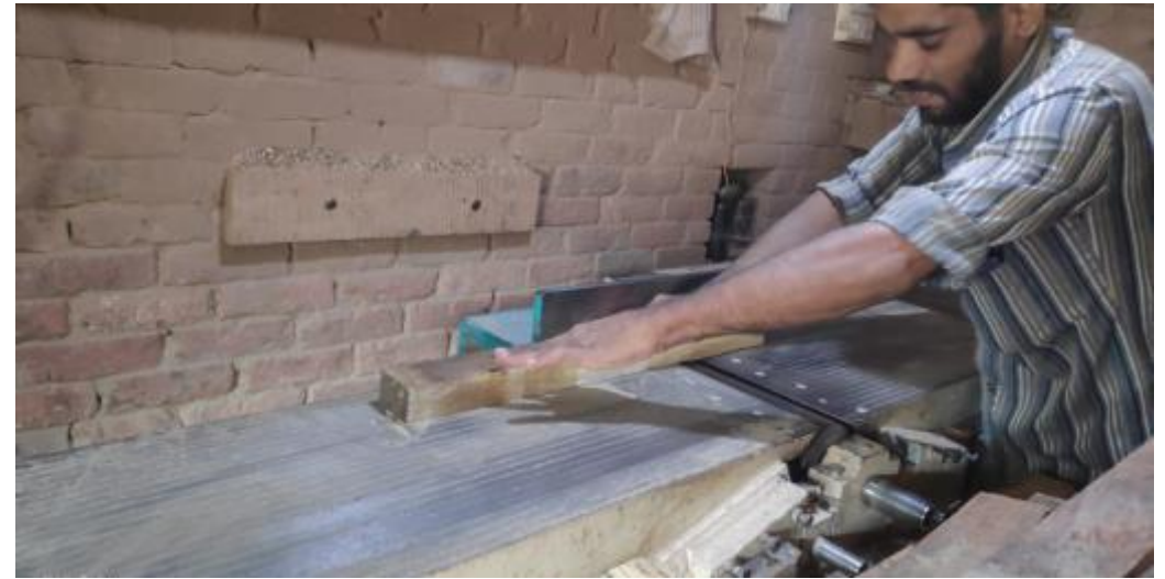
Leveling and cutting of in required shape
